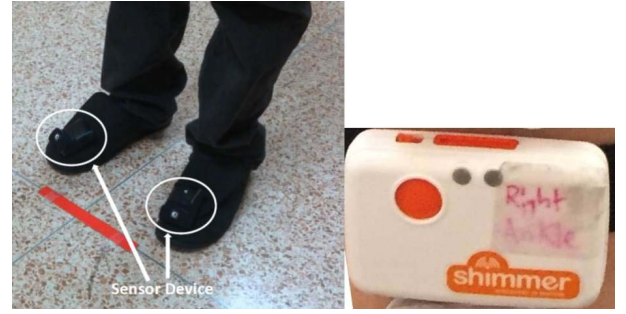
Fig. 3. Clinical setting used for data recording in glaucoma trial, consisting two shimmer sensors mounted on each shoe.
