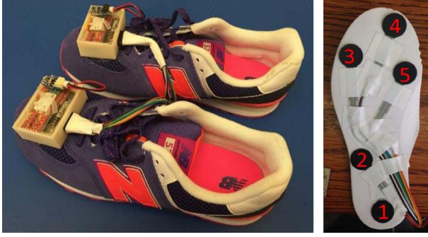
Fig. 4. Clinical setting of the shoe-integrated platform used for data recording in Rett trial, consisting accelerometer, gyroscope and pressure sensors in each shoe.
